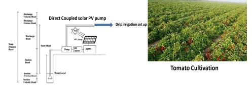
Fig. 1. Layout of the experimental study for solar PV water pumping based drip irrigation system in tomato cultivation.
